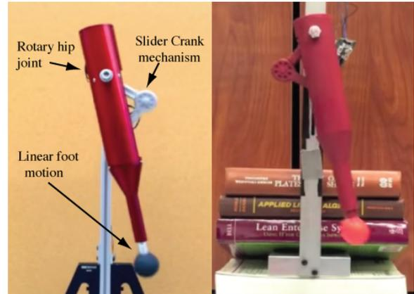
**Figure 1:** Modular robotic leg: Left: Machined from aluminum; Right: 3D printed. This one is half the size of the one shown on the left.
