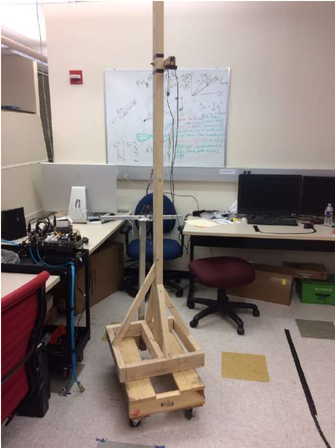
Figure 3 Sensor Testing Jig on Roller
