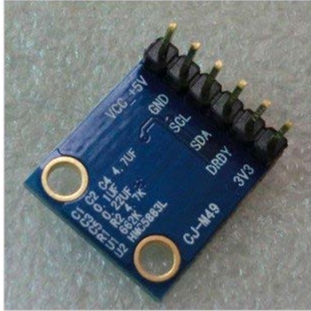
Fig 9. View of the pins on the HMC588L Magnetometer Sensor
